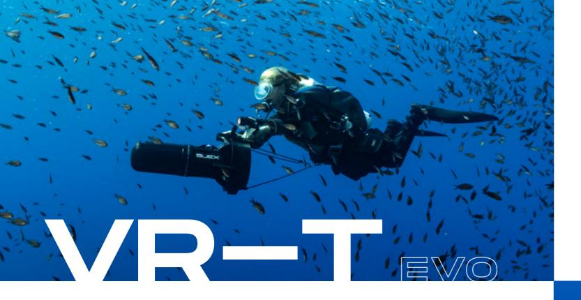
The VR-T EVO model is equipped with a NimH battery that can be charged in 4,5 hours and that allows up to 100 minutes runtime at a cruising speed or 60 minutes at a 65 m/min maximum speed.
