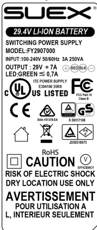
The battery charger is marked with a label on the bottom, which shows the technical data.
